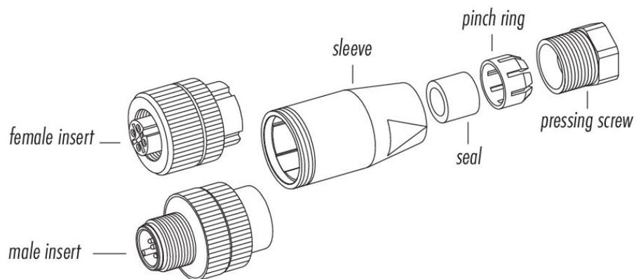
material of locking rings: zinc diecast, stainless steel
