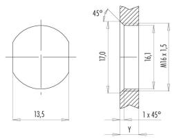
Installation direction: o-ring sits on chamfer.
