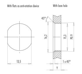
Installation direction: o-ring sits on chamfer.
