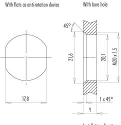
Installation direction: o-ring sits on chamfer.
