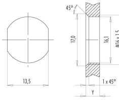
Installation direction: o-ring sits on chamfer.
