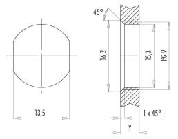
Installation direction: o-ring sits on chamfer.
